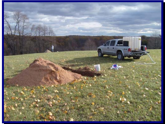
Hagerty provides stormwater management testing and design services, such as stormwater infiltration testing (shown above), in support of a Low Impact Development (LID) process. Subsequent services include subsurface infiltration BMP design
