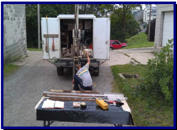
Subsurface investigation to evaluate soil impacts around a known underground storage tank (UST)
