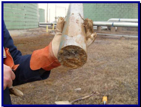
Undisturbed sample collected from emergency containment structure for permeability compliance
